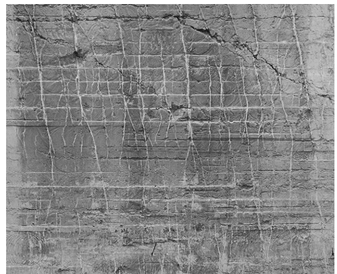
Fig. 7. Examples of layered carbonate fractured rocks: Quaternary marine bioclastic calcarenites (Salento, Southern Italy). The horizontal layering is partly masked by the quarry cuts; the width of the picture is about 5 m (Photo by U. Fracassi). Geological, tectonic and stratigraphic settings suggest a hydrostatic to sub-hydrostatic pore-fluid pressure ( \lambda_e \leq 0.4 ) and a low strength value ( |T_0| < 1\text{--}2 MPa) in agreement with the numerical results (Figs. 3a, b and 4b, c).
